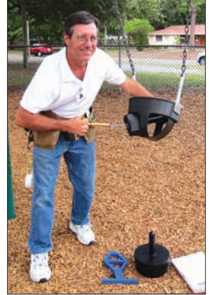
THIS TOT SEAT OPENING PASSES THE PULL TEST FOR A HANGING HAZARD — Photograph by the Author
